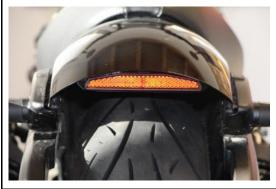
Stick the entire bracket to the fender centrally and flush at the rear and press on strongly.
