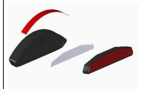
Caution: Lubricants are used to produce the part, so thoroughly clean and degrease the adhesive surface with brake cleaner.
